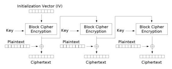
In practice, the keystream of the OFB mode can be seen as the one-time pad that is used to encrypt a message. This implies that in OFB mode, if the key and the IV are both reused, there is no security.
