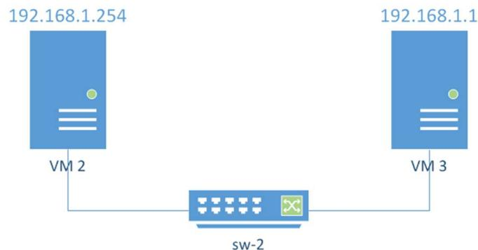
Diagram 3 - Expected layout of the subnet in which VM2 and VM3 will communicate using sw-2.
