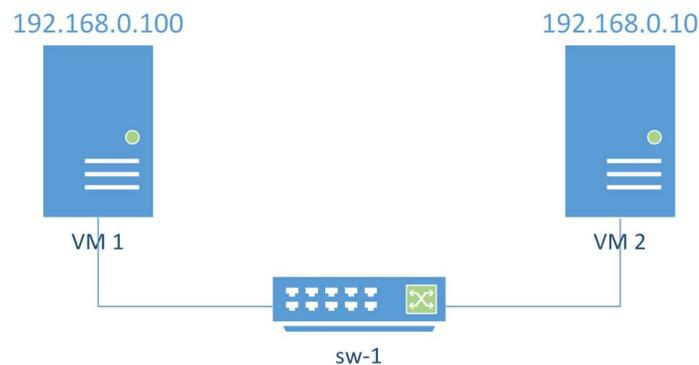
Diagram 2 - Expected layout of the subnet in which VM1 and VM2 will communicate using sw-1.
